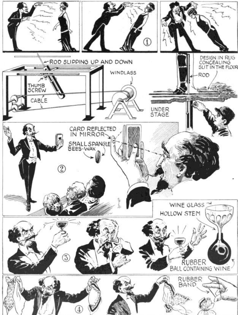
The Hypnotic Stunt (1) is Performed with Apparatus Shown. The Rod Slipped Through Tube, Operated by Windlass Beneath Stage, is Attached to the Lady's Legs. (2) To Read the Deck from the Back Use Small Mirror and Wax. (3) The Mystic Wineglass Fills as Soon as Emptied if Bulb is Pressed. (4) The Handkerchief's Knot When Thrown, with the Aid of a Rubber Band, Operator Snaps Band Over Corners When He Drops Them.
